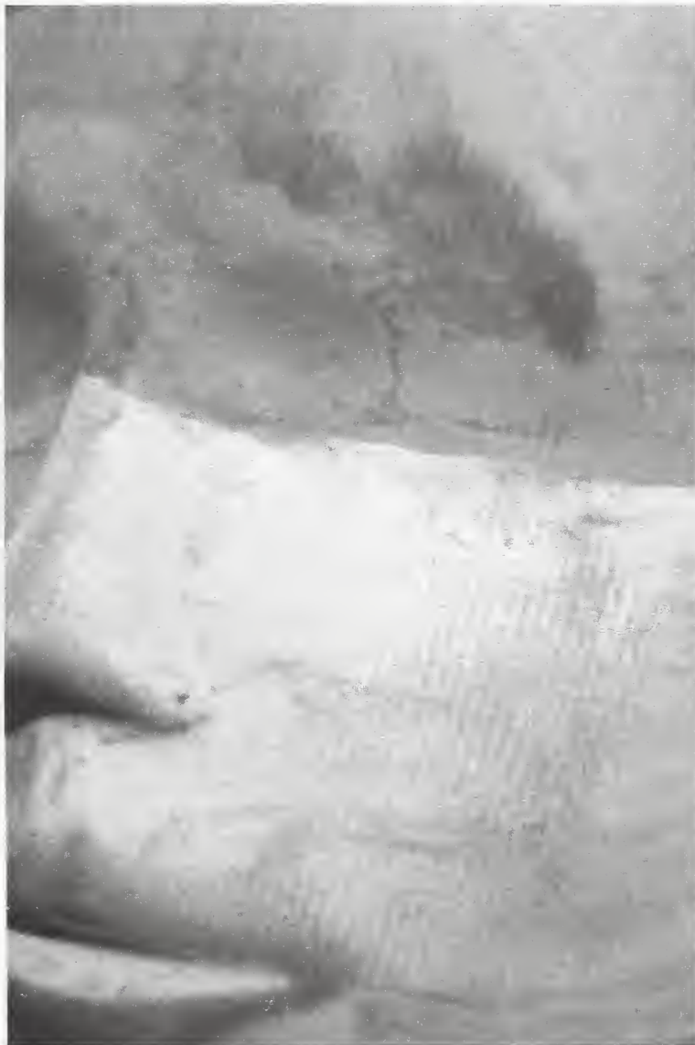
FIGURE 19 -- Close-up of Bag Imprints for Initially Positioned System D
